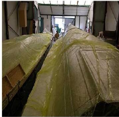
Vacuuming the outer skin laminate
